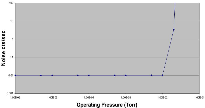
5 Micron Pore Chevron MCP Detector Noise vs. Operating Pressure
